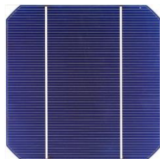
Figure 5: Cellule en Si monocristallin [9]
