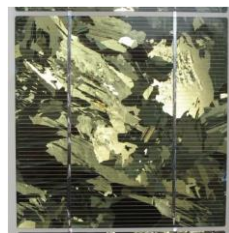
Figure 6: Cellule en Si poly-cristallin [9]
