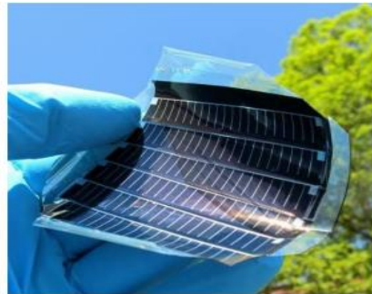
Figure (I-7) : Cellule CdTe [9]
