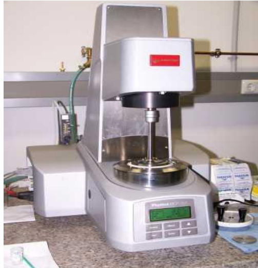
Figure 9 : Le RHEOPLUS/32 (Anton Paar) model MCR 301
