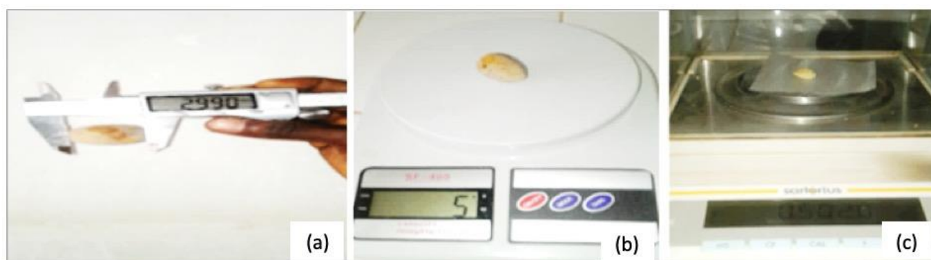
Figure 3: Measurement of dimensions and mass: using a sliding rule (a), a precision balance (b) and a Sartorius balance (c)
