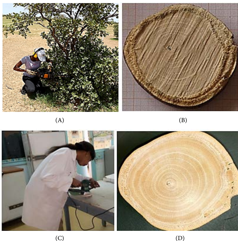
Figure 4. Picking and preparation of washers. (A) Washer pickup with a motorized chainsaw; (B) Example of washer removed; (C) Washer preparation with an orbital sander; (D) Washer after preparation.
