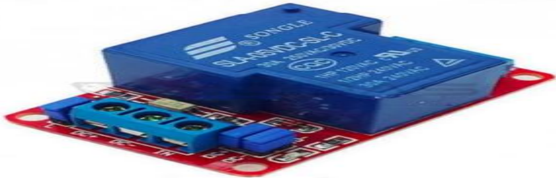
Figure IV.18 : Relais SONGLE SLA-05VDC-SLC
