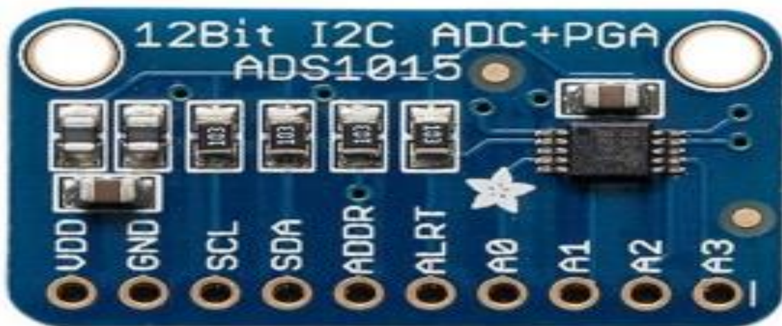
Figure IV.20 : Module i2C ADS1015 [20].
