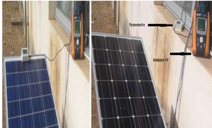
Figure 2. The mono and poly module under test with the I-V analyzer.
