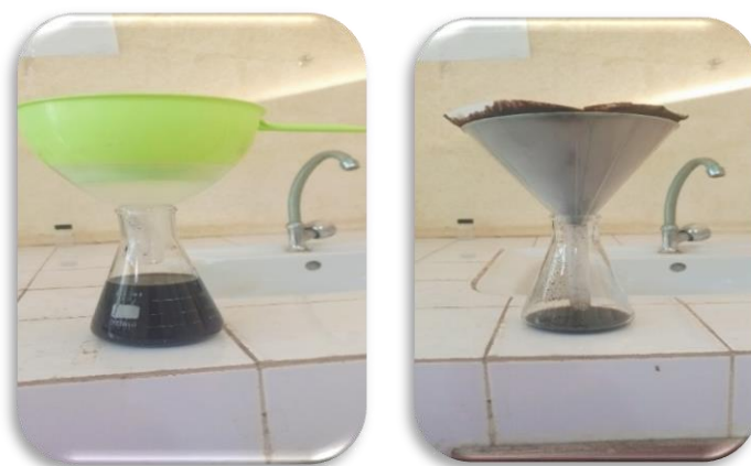
Figure 60 : dispositif de filtration (photo Ndeye Fatim FALL)
