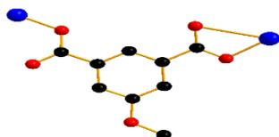
**Figure I.11** : Mode de coordination  $\mu_2$  monodentate et bidentate chélatant  $(\eta^1-\eta^0-\mu_1)-(\eta^1-\eta^1-\mu_1)-\mu_2$ .
