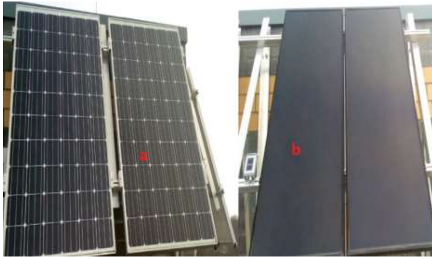
Figure 2. The technology crystalline silicone (a) and amorphe silicone (b) in field exposed for 5 years.
